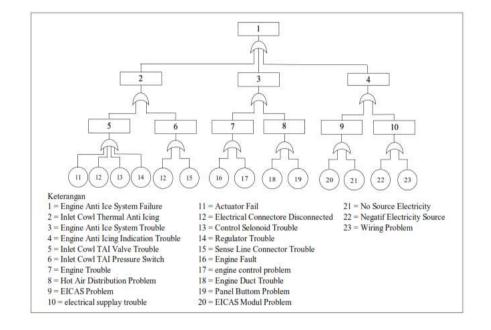
After making the FTA above, the next step is to determine the Minimum Cut Set (MCS) for the anti-ice system engine failure which is explained by Boolean algebra, as follows:
